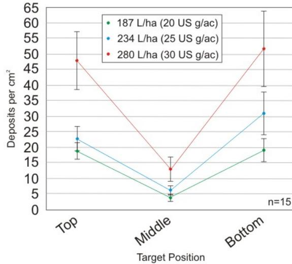
Figure 4: Combined average deposits per cm<sup>2</sup> for five different nozzle types at 187 L/ha (20 US g/ac), 234 L/ha (25 US g/ac) and 280 L/ha (30 US g/ac) at a ground speed of 16 kph (10 mph). Bars represent standard error.
