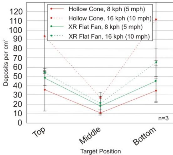
**Figure 8: Average deposits per cm<sup>2</sup> for Hollow cone and XR flat fan nozzles at 280 L/ha (20 US g/ac) and either 8 kph (5 mph) or 16 kph (10 mph). Bars represent standard error.**
