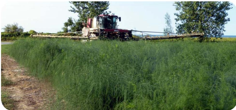
Figure 2: Self-propelled, front-mounted boom sprayer in asparagus in fern
