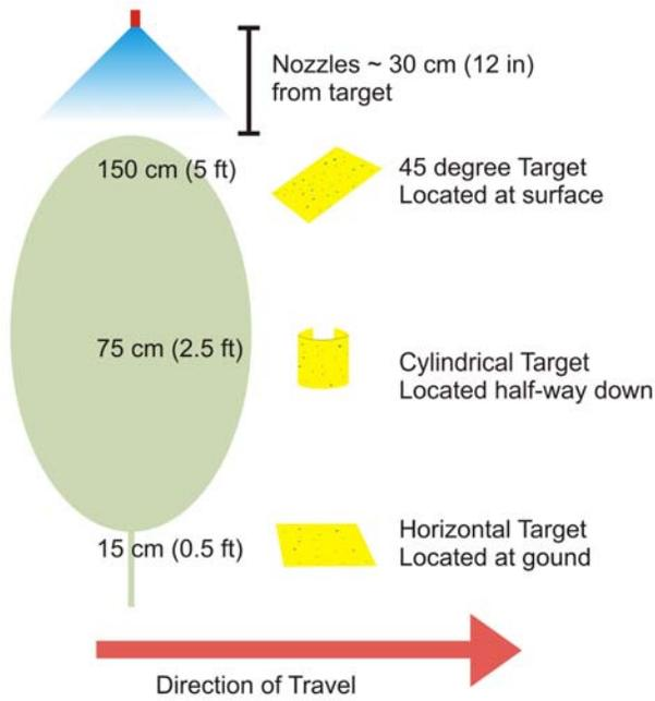
Figure 3: Layout of water-sensitive paper targets relative to asparagus fern, sprayer and sprayer direction of travel.
