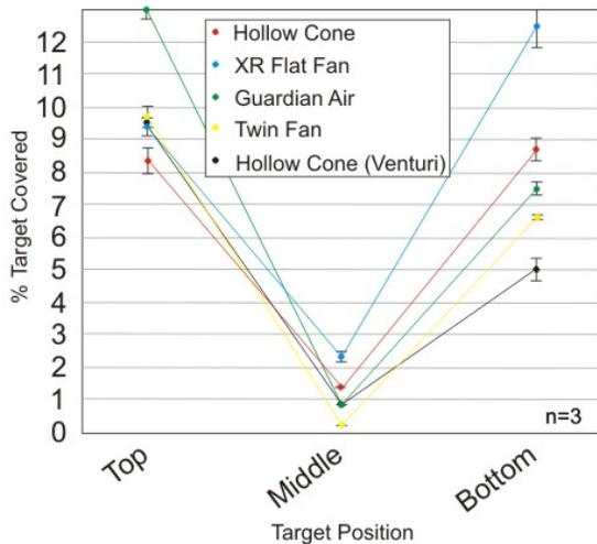
Figure 7: Average percent coverage for five different nozzle types at 280 L/ha (30 US g/ac) and 16 kph (10 mph). Bars represent standard error.
