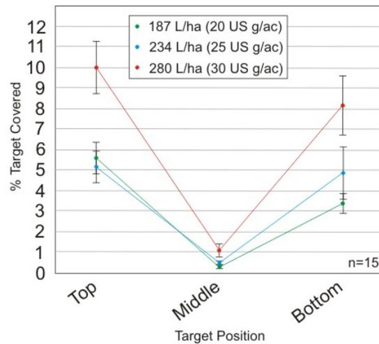
Figure 5: Combined average percent coverage for five different nozzle types at 187 L/ha (20 US g/ac), 234 L/ha (25 US g/ac) and 280 L/ha (30 US g/ac) at a ground speed of 16 kph (10 mph). Bars represent standard error.
