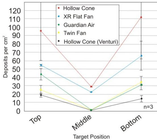
Figure 6: Average deposits per cm<sup>2</sup> for five different nozzle types at 280 L/ha (30 US g/ac) and 16 kph (10 mph). Bars represent standard error.
