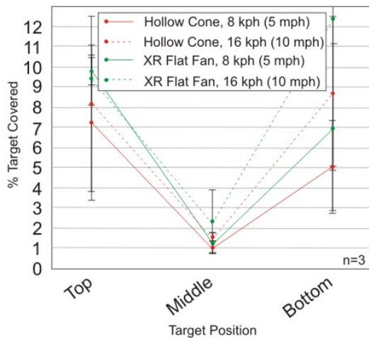
**Figure 9: Average percent coverage for Hollow cone and XR Flat fan nozzles at 280 L/ha (30 US g/ac) and either 8 kph (5 mph) or 16 kph (10 mph). Bars represent standard error.**
